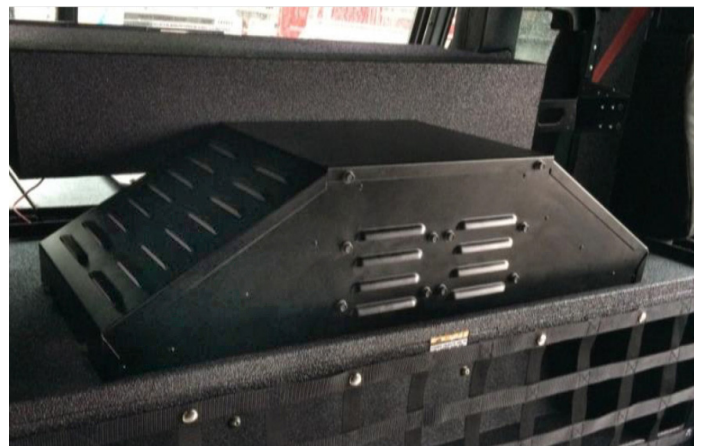
HEPA filtration system for cab interior
